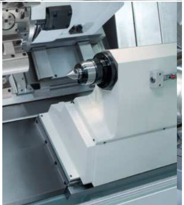
'B' axis tailstock (Standard on B750 / Option on B1250).
